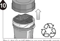
The Lubri-Cup VG Mini is an eco-friendly product that can be disposed of separately. Turn the housing cap counterclockwise to disassemble the product for proper disposal.
