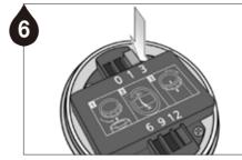
Firmly push the Mode Selector into the slot of the desired period.
